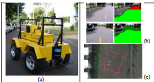
Fig. 1. (a) Mechanical structure of the outdoor robotic vehicle (b) Experimental validation: GPS waypoint trajectory following (bottom); Image based obstacle detection (top)
